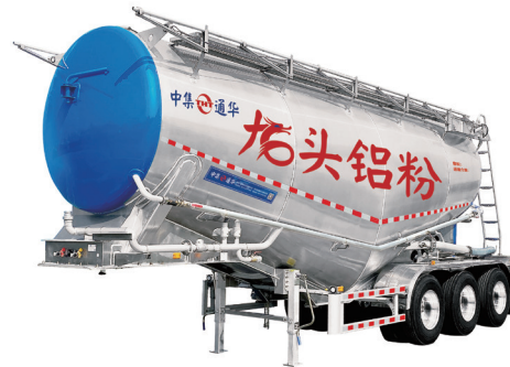
Intelligent Aluminum Alloy Horizontal Dry Bulk Tank Trailer
