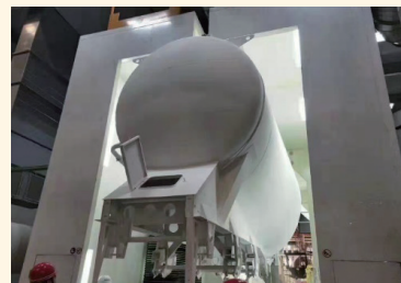
Powder Spraying Workshop for Liquid Tank Trailers
