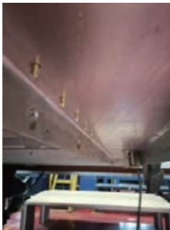
113.1db of noise released in case of pneumatic tool with aluminum solid rivet, with a peak of 125db
