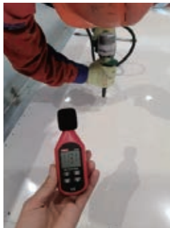
113.1db of noise released in case of pneumatic tool with aluminum solid rivet, with a peak of 125db
