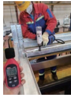
Riveting by the riveting tool using blind rivets, with a peak of 85.8db
