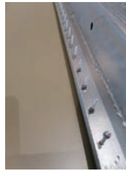
Riveting by the riveting tool using blind rivets, with a peak of 85.8db
